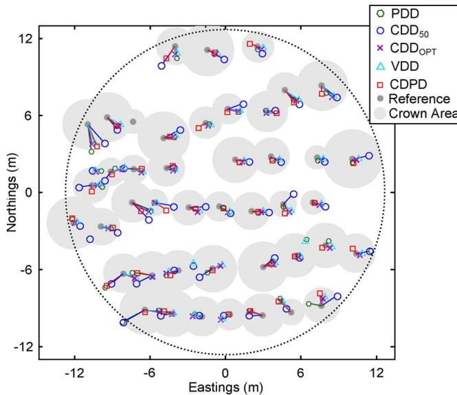
Fig. 5. Distribution of tree location errors over plot 6 using full-scale data within the five algorithms analyzed.
