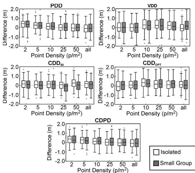
Fig. 6. Box plot (showing the 5th, 25th, 50th, 75th, and 95th quartiles) showing the difference between field and LiDAR measured crown widths of isolated trees and trees in small groups for each algorithm and at each density.
