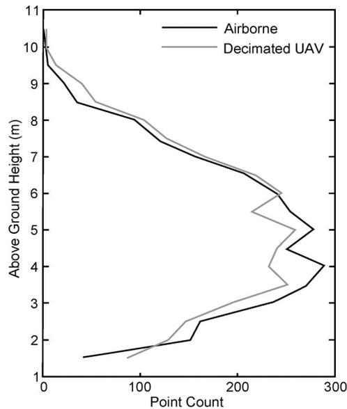
Fig. 1. Above ground height distributions of full-scale airborne and UAV data decimated to the same density ( $8 \text{ p/m}^2$ ) captured over a coincident area.
