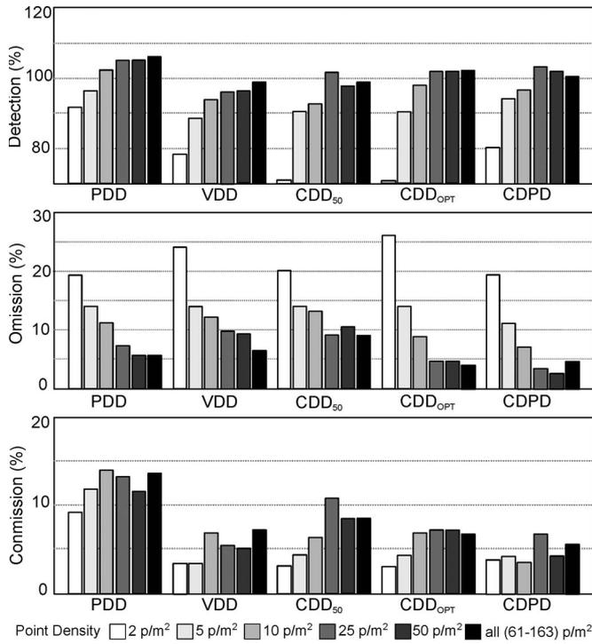
Fig. 3. Detection, omission, and commission rates for the five algorithms utilizing the five different point densities. There was a total of 272 trees within 5 plots.
