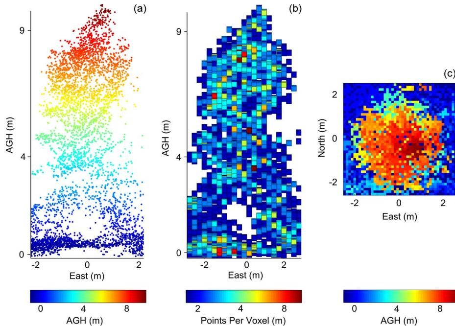
Fig. 2. Representation of the three feature spaces: (a) the original point cloud; (b) 0.2-m cubic voxel space; and (c) a 0.1-m-resolution CHM, analyzed in this paper as derived from an unfiltered point cloud.
