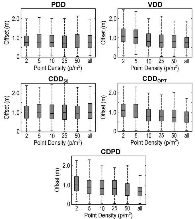
Fig. 4. Box plot (showing the 5th, 25th, 50th, 75th, and 95th quartiles) showing the absolute offsets between field and LiDAR measured tree locations for each algorithm and at each density.
