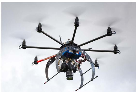
Fig. 1. OktoKopter in flight fitted with Canon 550D.
