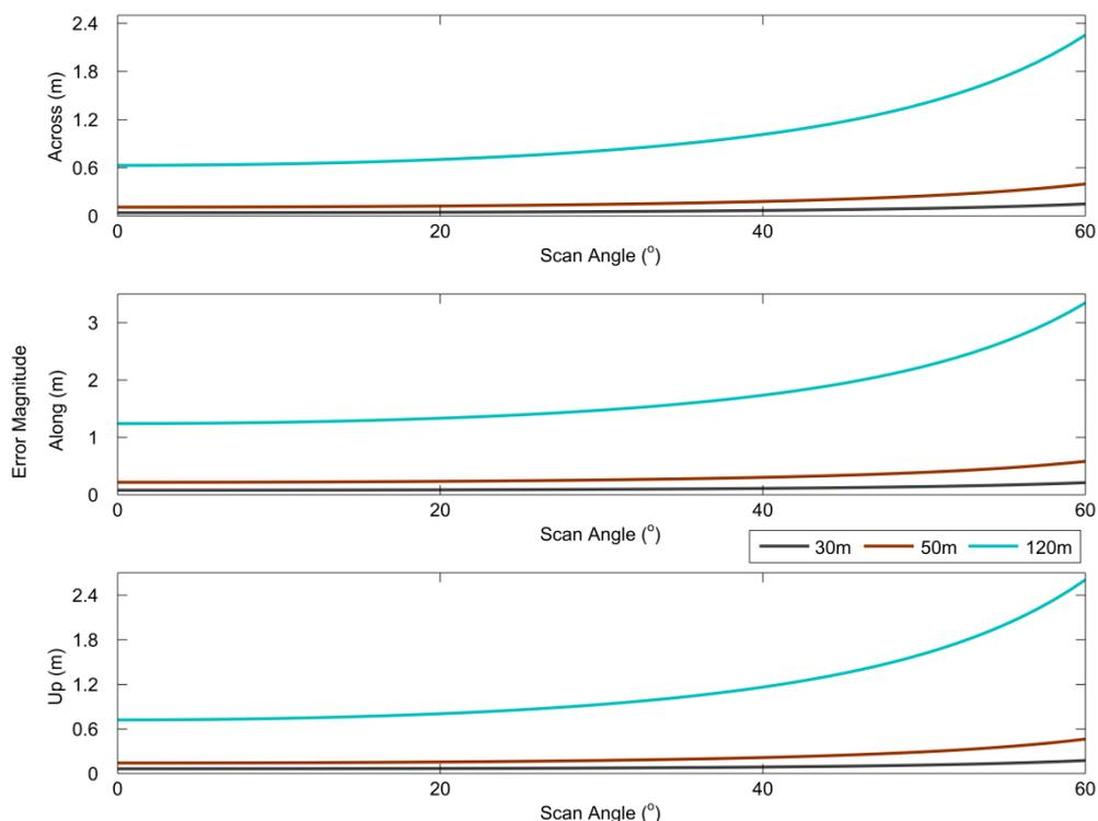
Figure 5. The accuracy of the TerraLuma LiDAR system based on the error statistic presented in Table 1 ( $\sigma_\omega$ ,  $\sigma_\phi$  and  $\sigma_\kappa = 0.35^\circ$ ) and at flying heights of 30 m, 50 m and 120 m.
