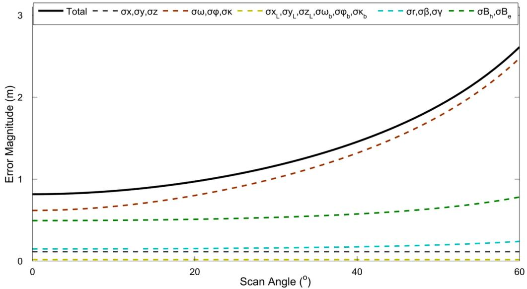
Figure 3. The result of a GPS/IMU filtering strategy constraining orientation error, to  $0.5^\circ$  in pitch and roll and  $1.5^\circ$  in Yaw, at a flying height of 40 m resulting in a higher overall LiDAR point positioning accuracy.
