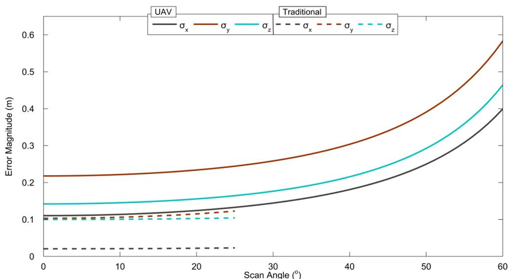
Figure 6. Accuracy of the TerraLuma LiDAR system ( $\sigma\omega$ ,  $\sigma\phi$  and  $\sigma\kappa = 0.35^\circ$ ) flying at 50 m in comparison to the accuracy of a traditional full scale system flying at 1100m (full scale system properties adapted from Goulden and Hopkinson, 2010).
